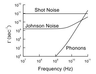
Figure 6: Scattering rates attributable to shot noise, Johnson noise and phonons. The value for  $\Gamma$  in Eq. 8 is plotted assuming M=1, i. e., coupling between states is maximal. Scattering arising from both shot noise and Johnson noise will roll of at high frequencies as a result of circuit capacitance, which has been neglected.
